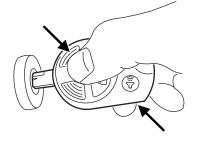
To gain more leverage when rotating the IKT in the ignition lock cylinder, you can readjust the location of your thumb to grasp the IKT on the outer edge next to the  $\square$  control.
